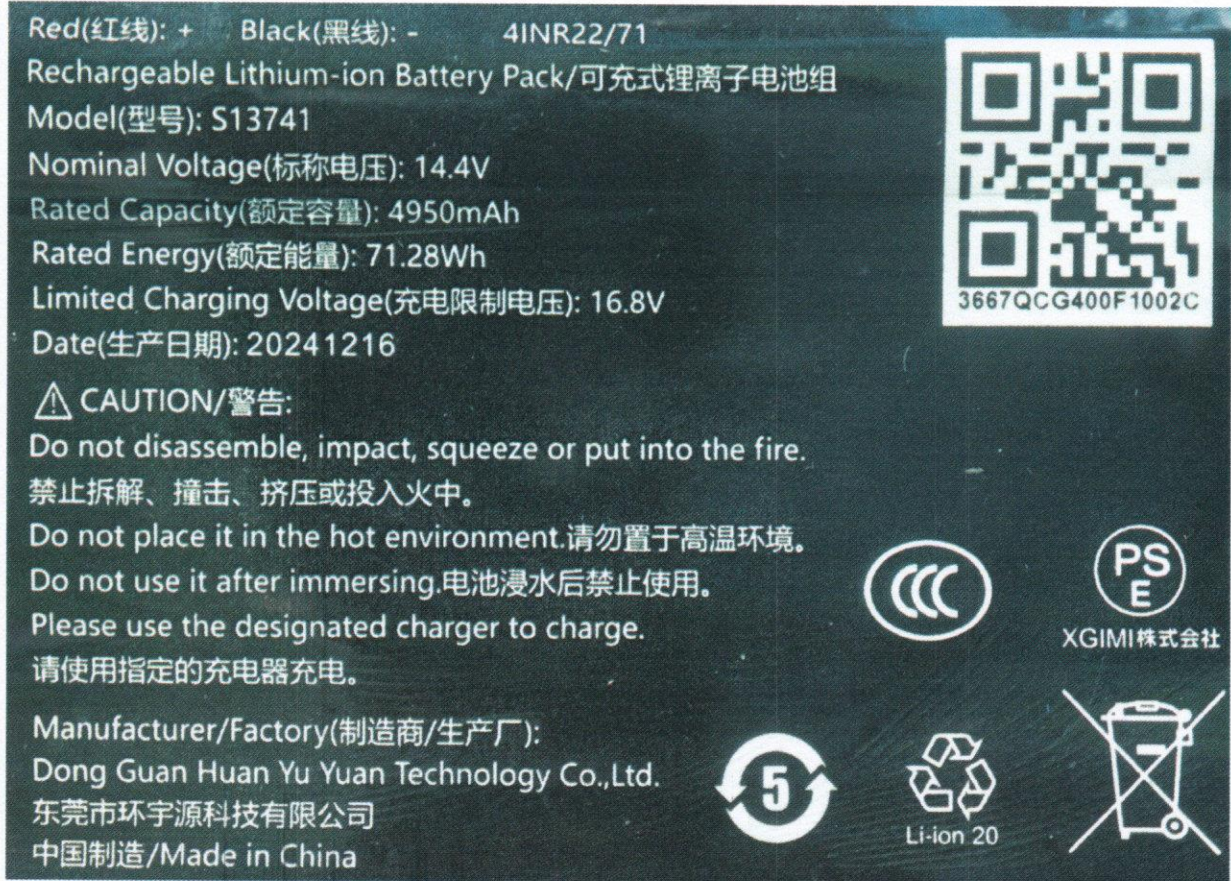
电池组铭牌 View of the battery nameplate
