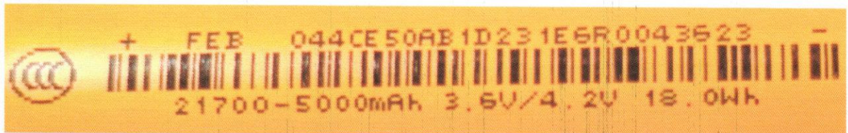
组成电池铭牌 View of the battery structure
