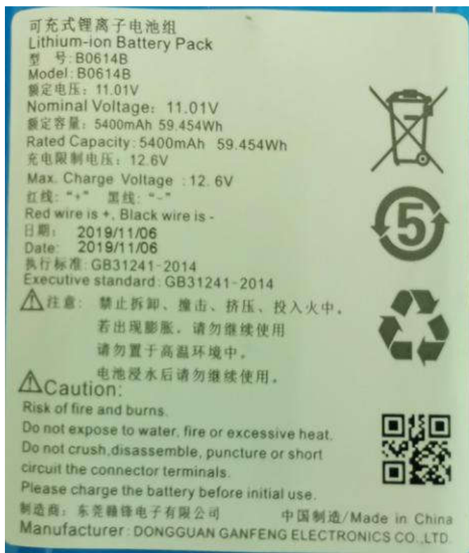
电池组铭牌 View of the battery nameplate
