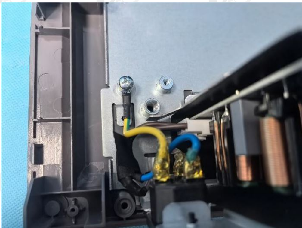
Internal view 15 (Protective earthing) for models XR06B and XR03B
